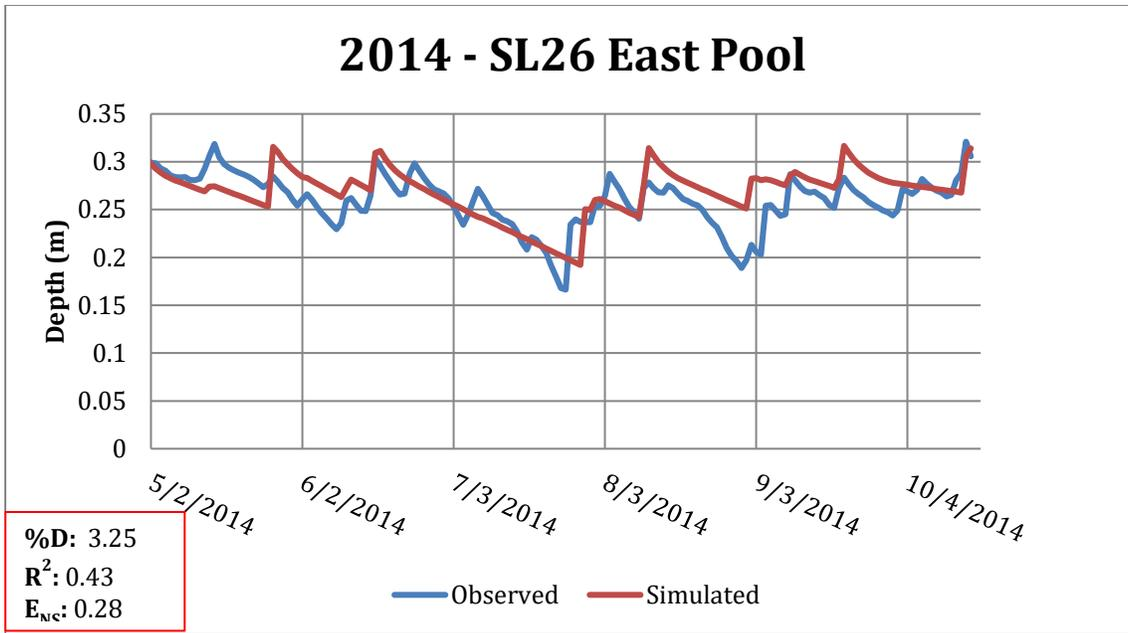
Figure 9: Sideline 26 East Pool Validation with 2014 data
