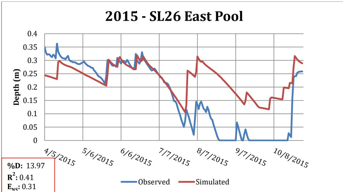
Figure 11: Sideline 26 East Pool Validation with 2015 data
