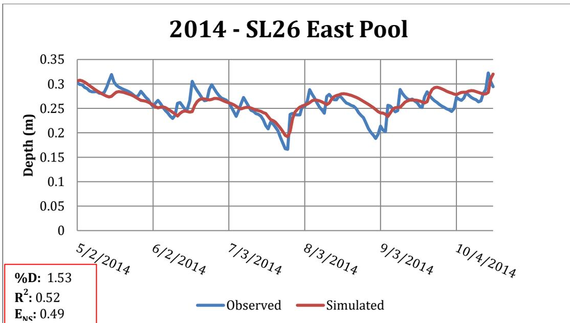
Figure 18: Sideline 26 East Pool Validation with 2014 data
