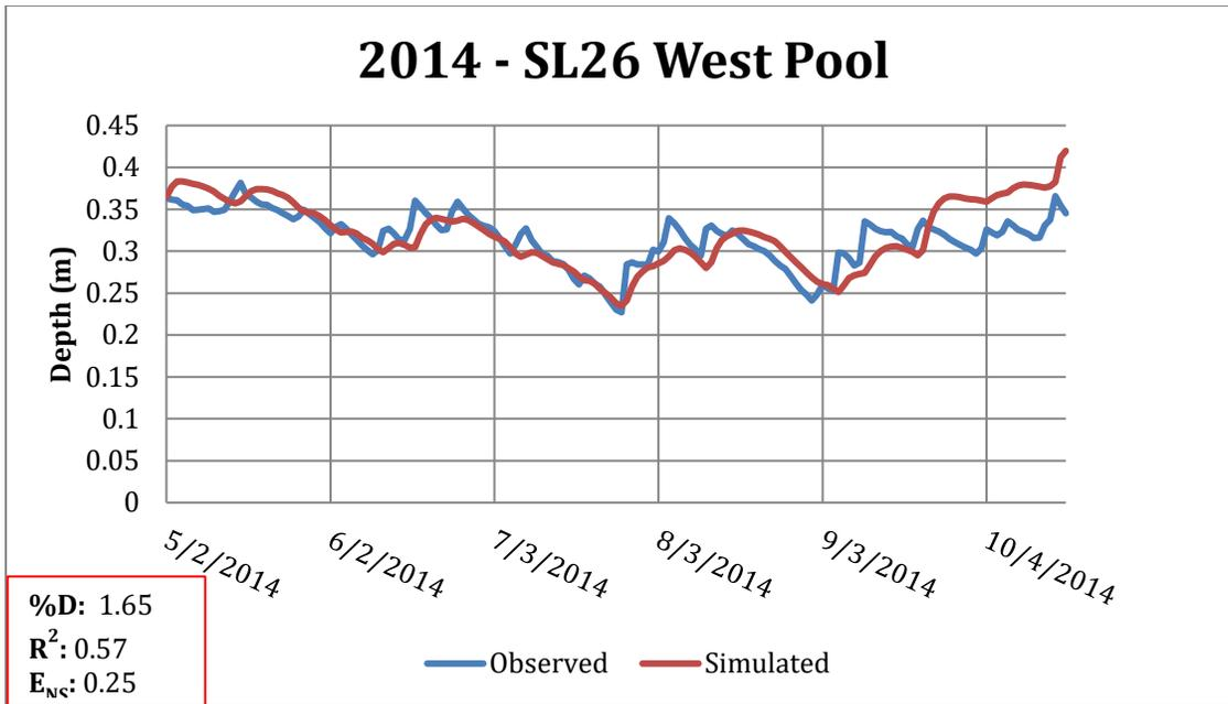
Figure 17: Sideline 26 West Pool Validation with 2014 data
