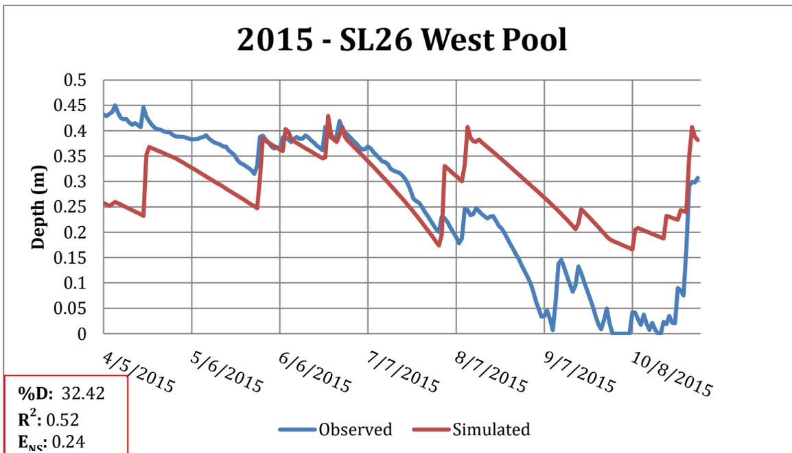
Figure 10: Sideline 26 West Pool Validation with 2015 data
