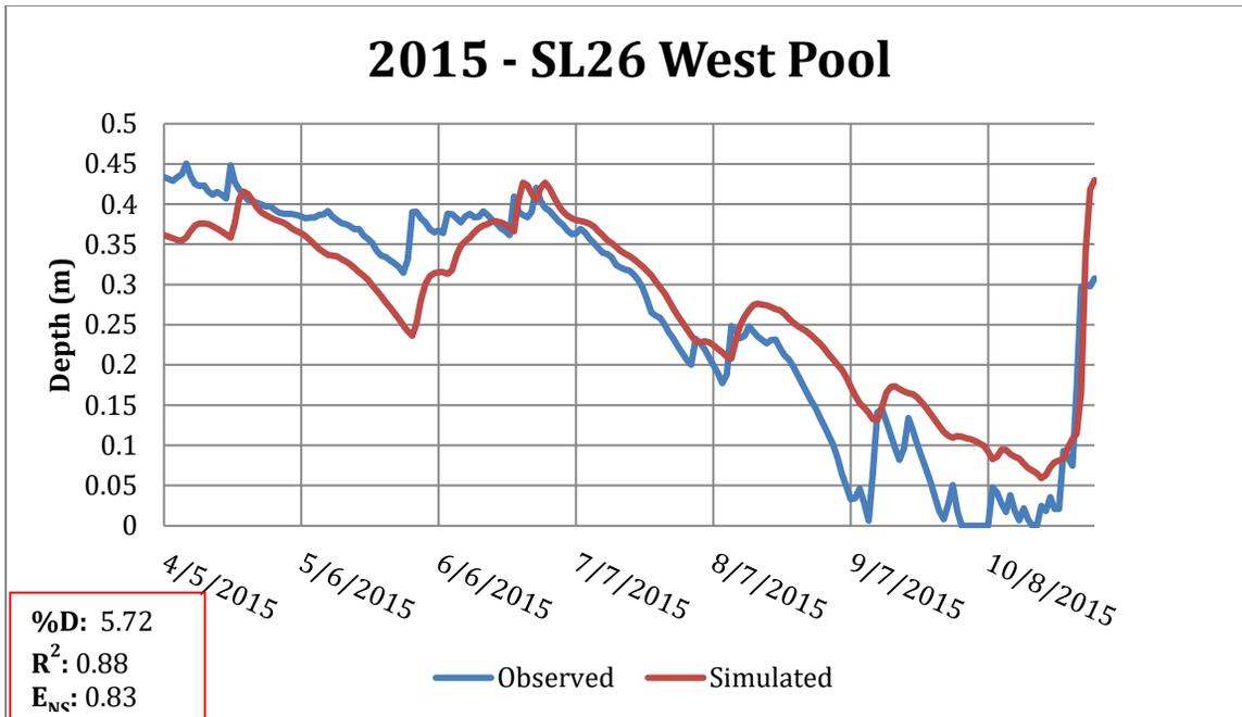
Figure 19: Sideline 26 West Pool Validation with 2015 data
