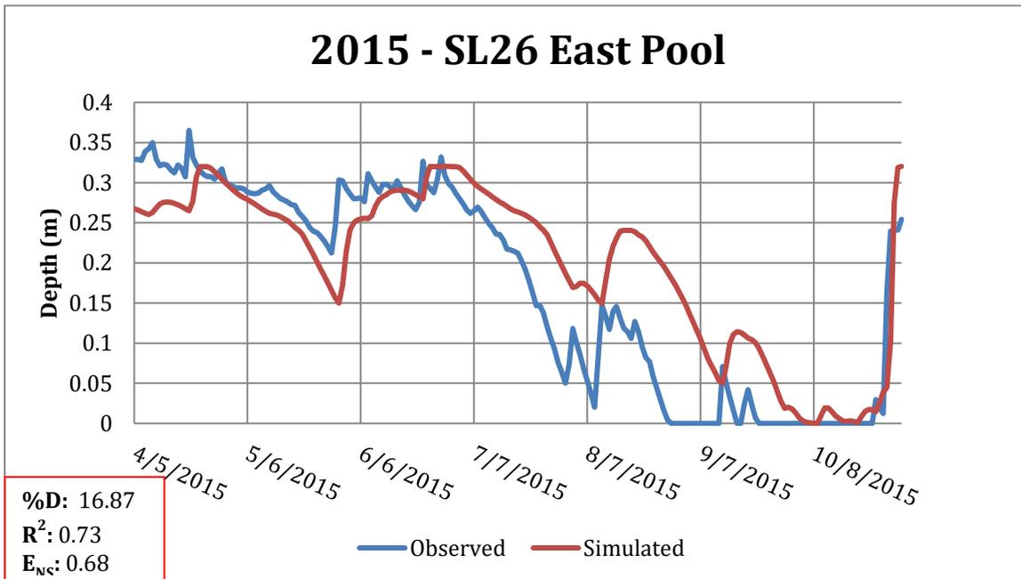
Figure 20: Sideline 26 East Pool Validation with 2015 data
