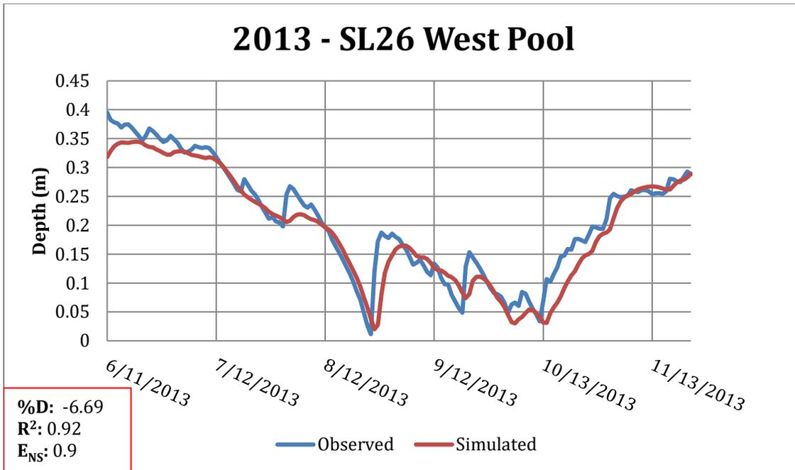
Figure 15: Sideline 26 West Pool Calibration with 2013 data
