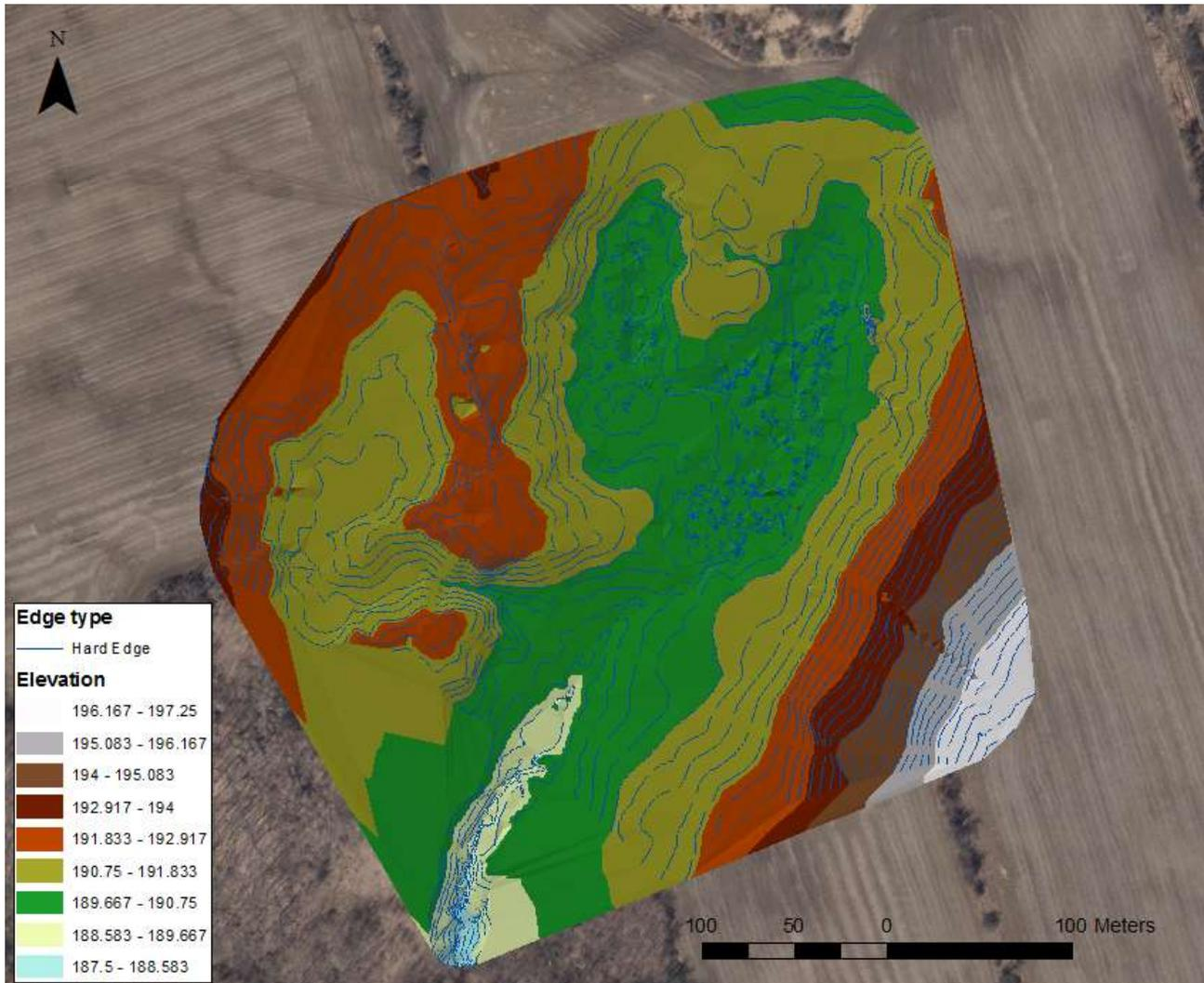
Figure 4: Sideline 26 Wetland Topography and Bathymetry
