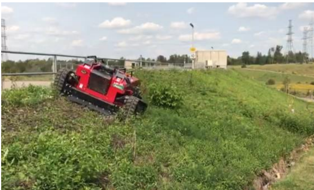
Figure 8 TRCA remote-controlled slope mower cutting the G. Ross Lord Dam embankment. This equipment allows very steep slopes to be maintained without putting staff at risk.
