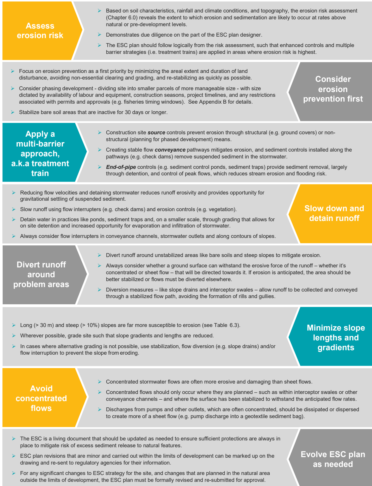
Figure 7.1: Principles of ESC planning
