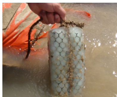
Figure B2-25: Polymer flocculant in gel-block form
