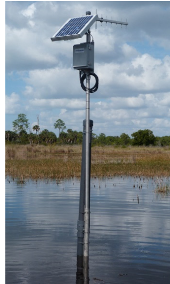
Figure 10.1: An in-water turbidity monitoring station.
