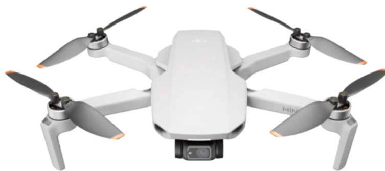
Figure 7.3 - Micro Remotely Piloted Aircraft System (mRPAS) (DJI Mini 2). Source: DJI, 2021.
