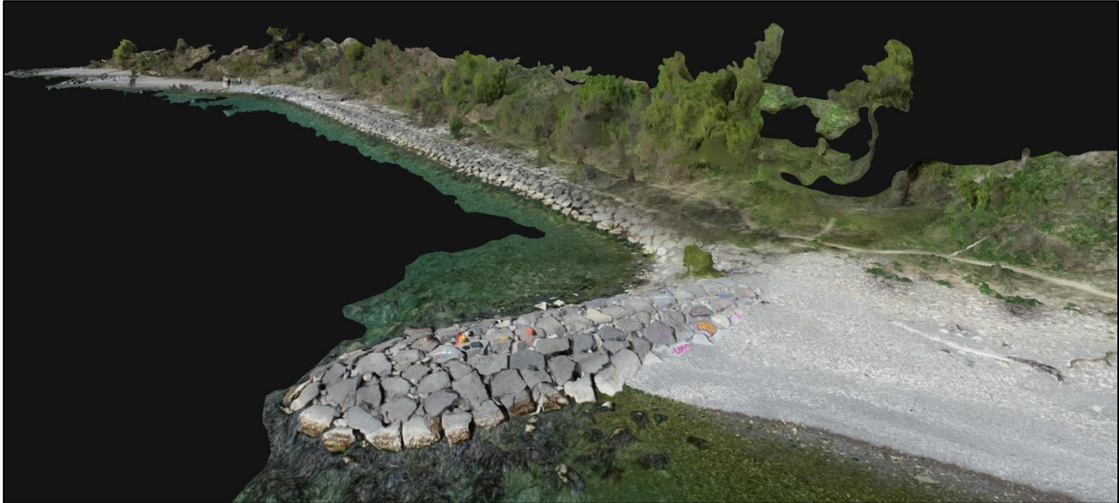
Figure 5.7 - Photogrammetric model a waterfront system at the toe of Lakehurst Crescent (WF20). Source: TRCA, 2021.
