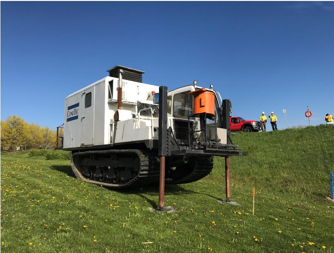
**Figure 7** Stouffville Dam undergoing earthquake liquefaction investigation.
