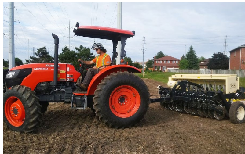
Figure 23: Seed drills are advantageous for their even distribution of seeds but do require packed, flat and relatively dry soil.
