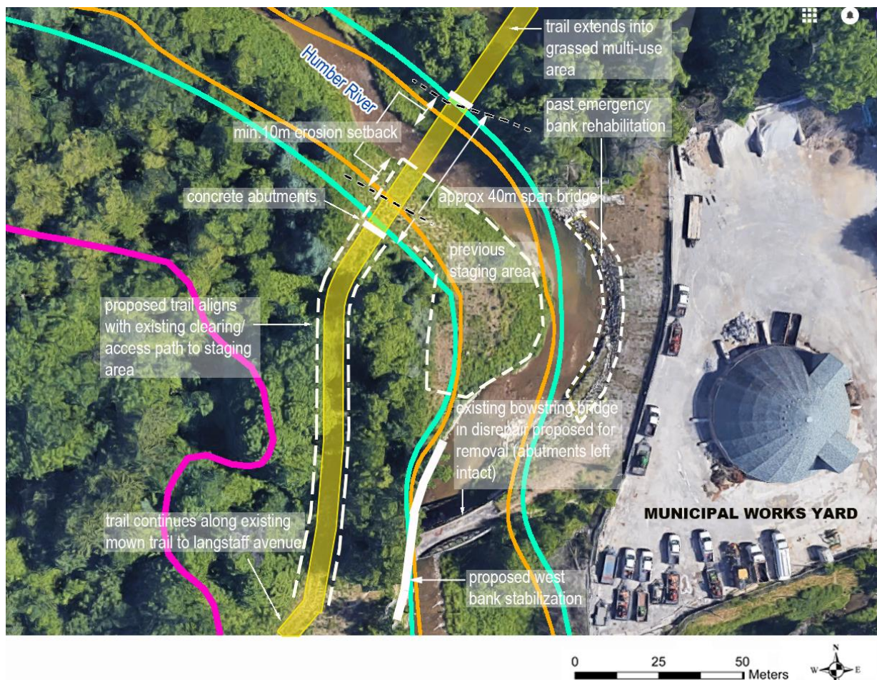
Figure 6: Focus Area 2 Concept Plan Enlargement
