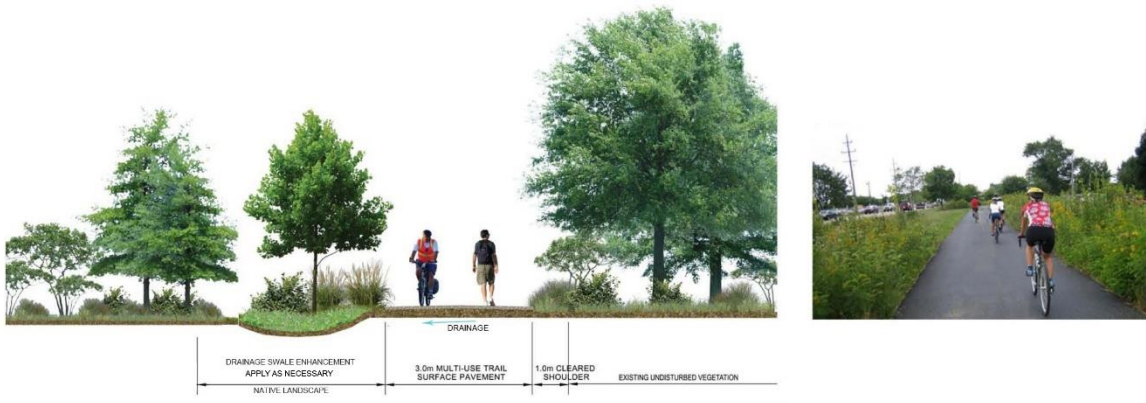
Figure 35: Typical Asphalt Multi-Use Trail Cross Section
