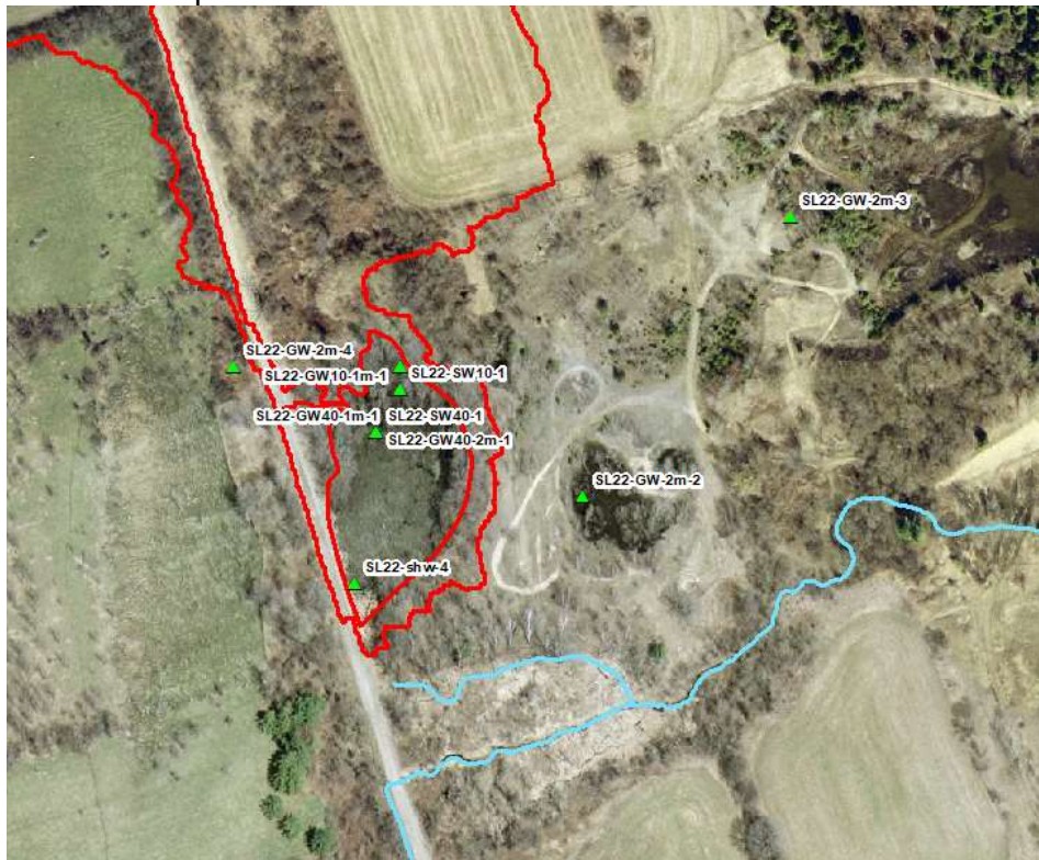
Figure 28: Location of water level monitoring wells at Sideline 22
