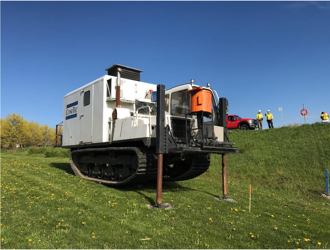
Figure 7 Stouffville Dam undergoing earthquake liquefaction investigation.
