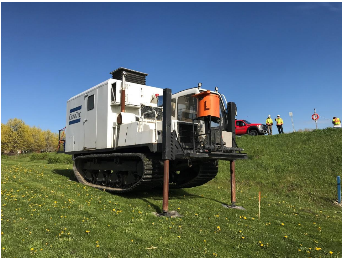
Figure 7 Stouffville Dam undergoing earthquake liquefaction investigation.
