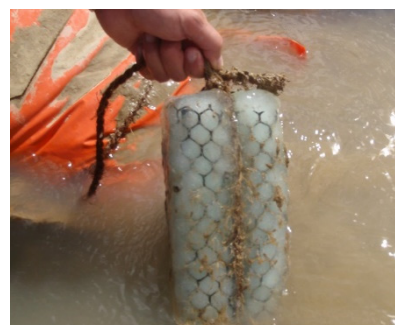
Figure B2-25: Polymer flocculant in gel-block form
