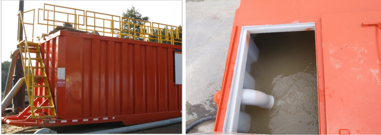
Figure B2-22: Weir tanks
