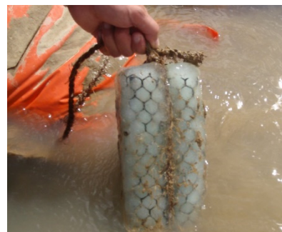
Figure B2-25: Polymer flocculant in gel-block form
