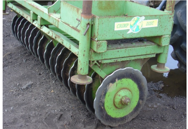
Figure B1-8: Straw crimper
