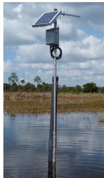
Figure 10.1: An in-water turbidity monitoring station.
