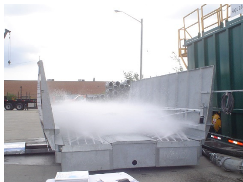
Figure B2-28: Vehicle tracking controls. From top to bottom: mud mat, shaker rack, vehicle wheel washer.
