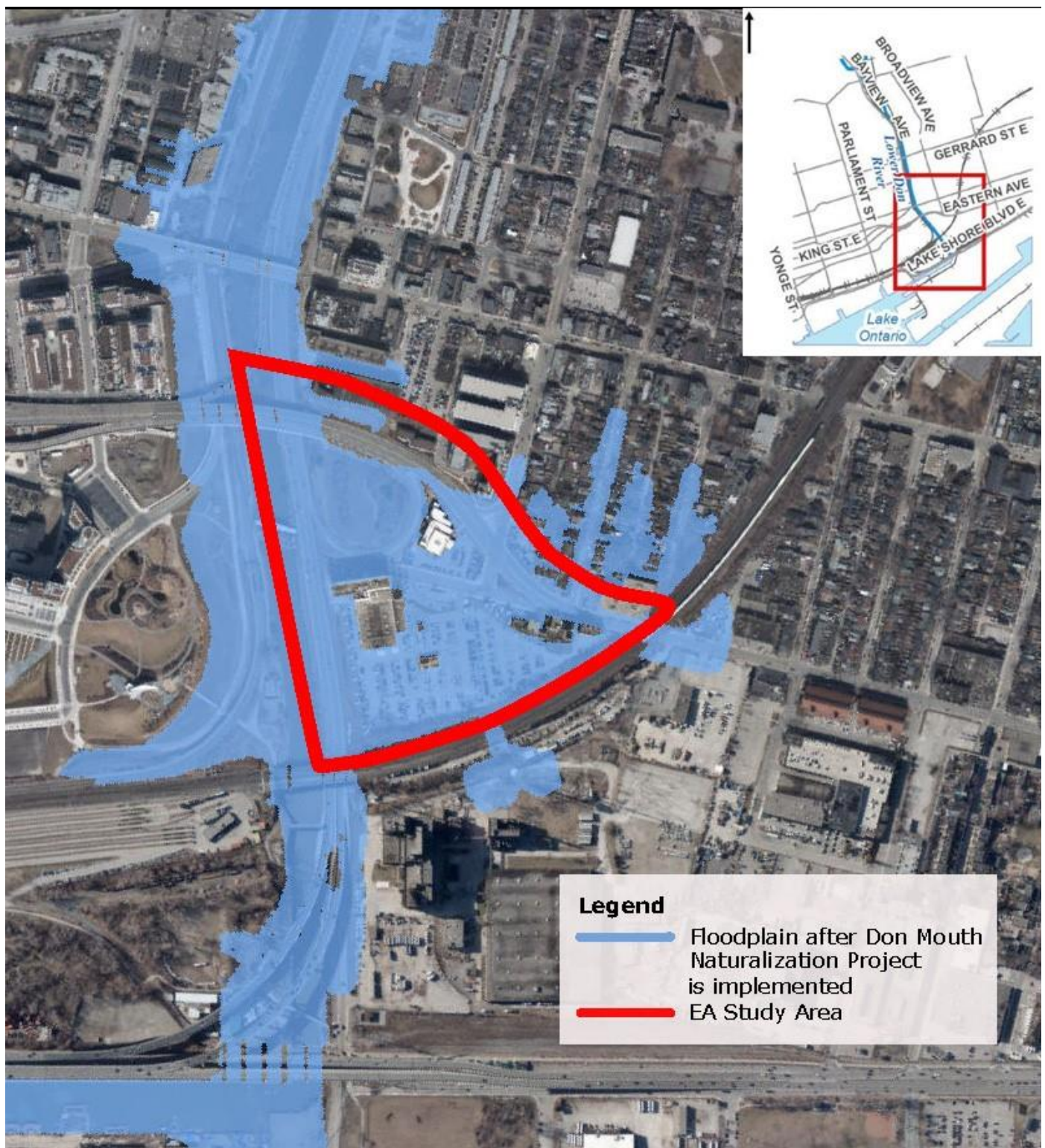
Figure 1. Residual flooding of urban lands during the regional storm event following full implementation of the Don Mouth Naturalization Project. The BEFP project study area is outlined in red within the inset map (top right). Note that the blue shading on the western side of the river is designed to hold water (it is the 'wet side' of a flood protection landform at Corktown Common).
