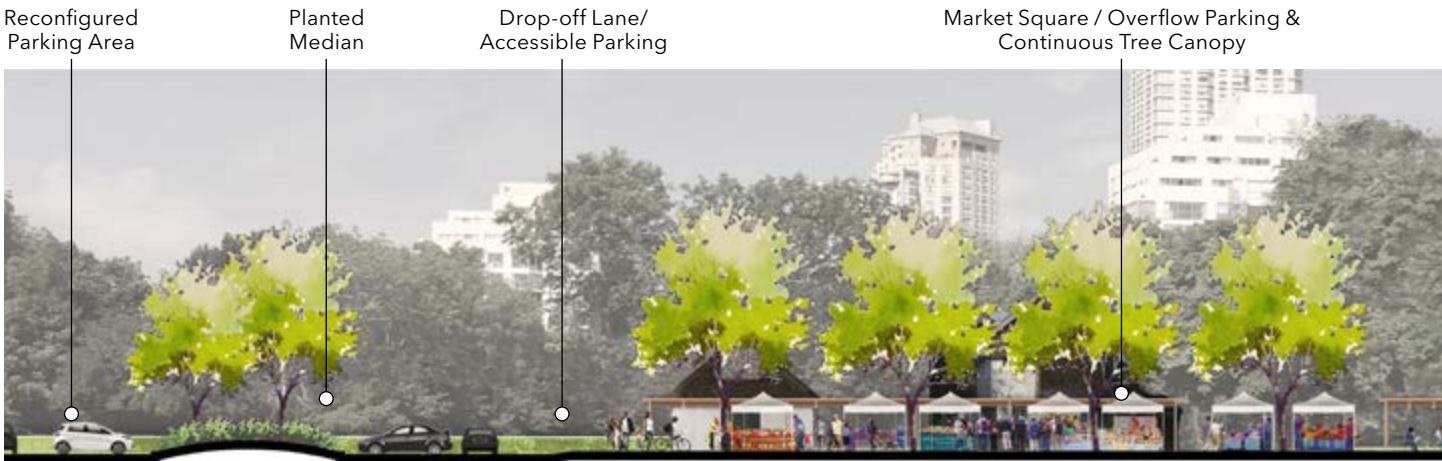
Section through the reconfigured western parking, highlighting new social and ecological spaces and the proposed adjustments in grade, planting and materials
