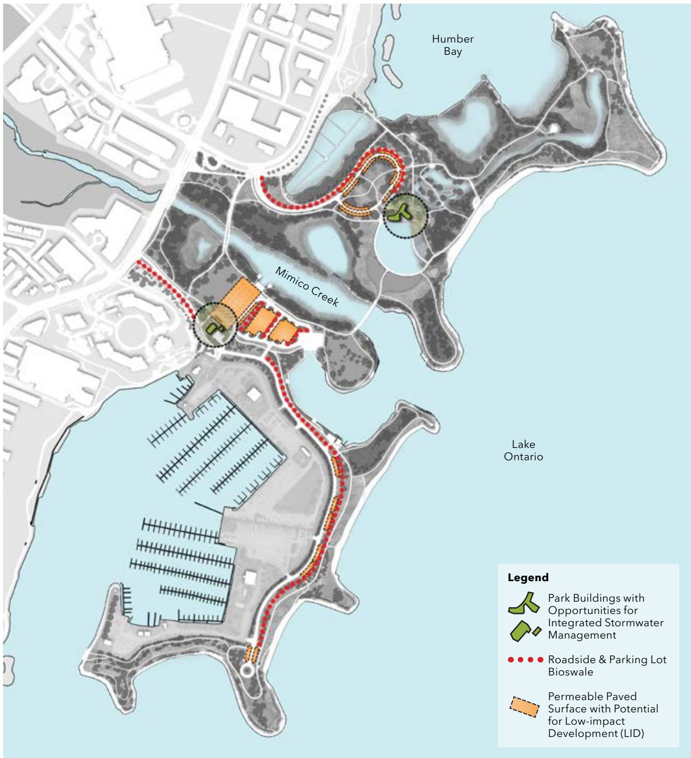
Potential improvements to the stormwater management system within Humber Bay Park
