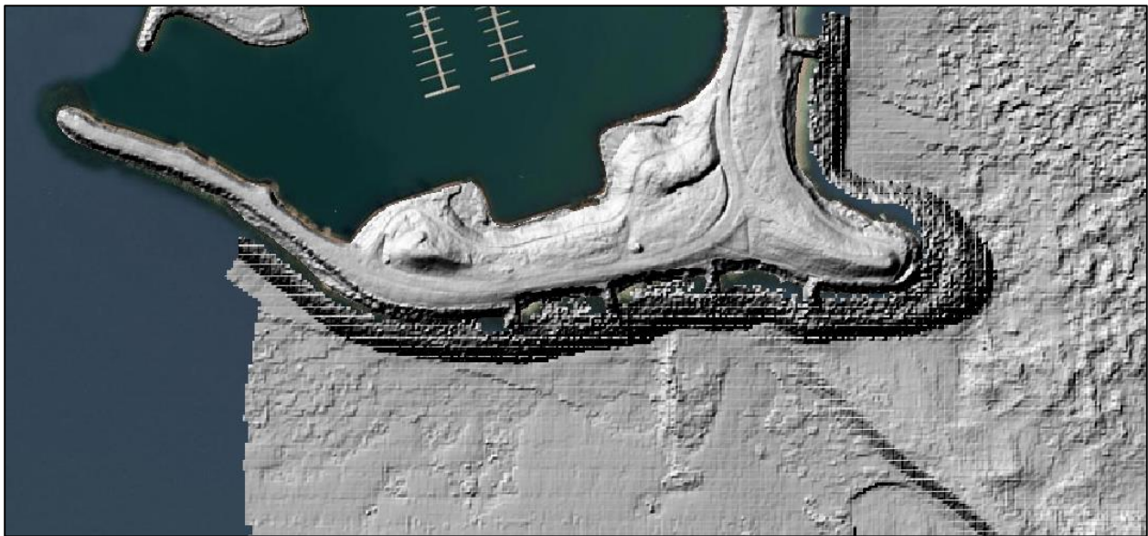
Figure 7.6 - Two merged Digital Surface Models (collected by RPAS for land, and by multibeam echo sounding for underwater) of the erosion control system at Colonel Sam Smith (WF04). Source: TRCA, 2022.
