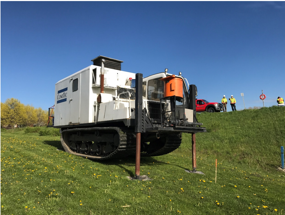
Figure 7 Stouffville Dam undergoing earthquake liquefaction investigation.
