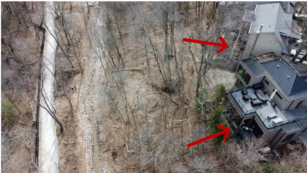
Figure 2. Drone photography of the slope failure facing southeast below 193 – 195 Hudson Drive. Red arrows highlighting 193 – 195 Hudson Drive. Trail to the left of the photo is the Beltline Trail. Source: TRCA 2018
